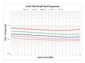
NOTE: Graph data was taken on a random sample using an Audio Precision Model APX555 Audio Analyzer.
